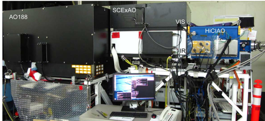
FIG. 2.—Image of SCEXAO mounted at the Nasmyth IR platform at Subaru Telescope. To the left is AO188, which injects the light into SCEXAO (center), and HiCIAO is shown on the right. The FIRST recombination bench is not shown for visual clarity. See the electronic edition of the PASP for a color version of this figure.
