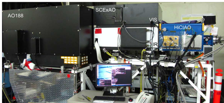
FIG. 2.—Image of SCEXAO mounted at the Nasmyth IR platform at Subaru Telescope. To the left is AO188, which injects the light into SCEXAO (center), and HiCIAO is shown on the right. The FIRST recombination bench is not shown for visual clarity. See the electronic edition of the PASP for a color version of this figure.
