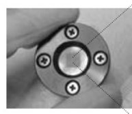
Figure 1: A picture and a scanning electron microscope image of a photonic-crystal coronagraphic mask. (manufactured by the Photonic Lattice, Inc.)
