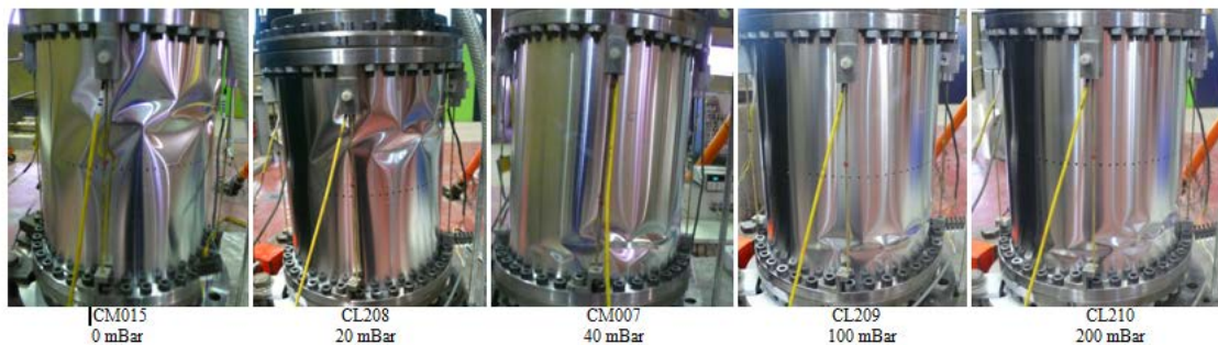
Figure 4-71. Effet de la pression - Modes critiques expérimentaux, PM, Aluminium, L/R = 2, R/t = 665, H/R = 13.54 (fibre neutre)
