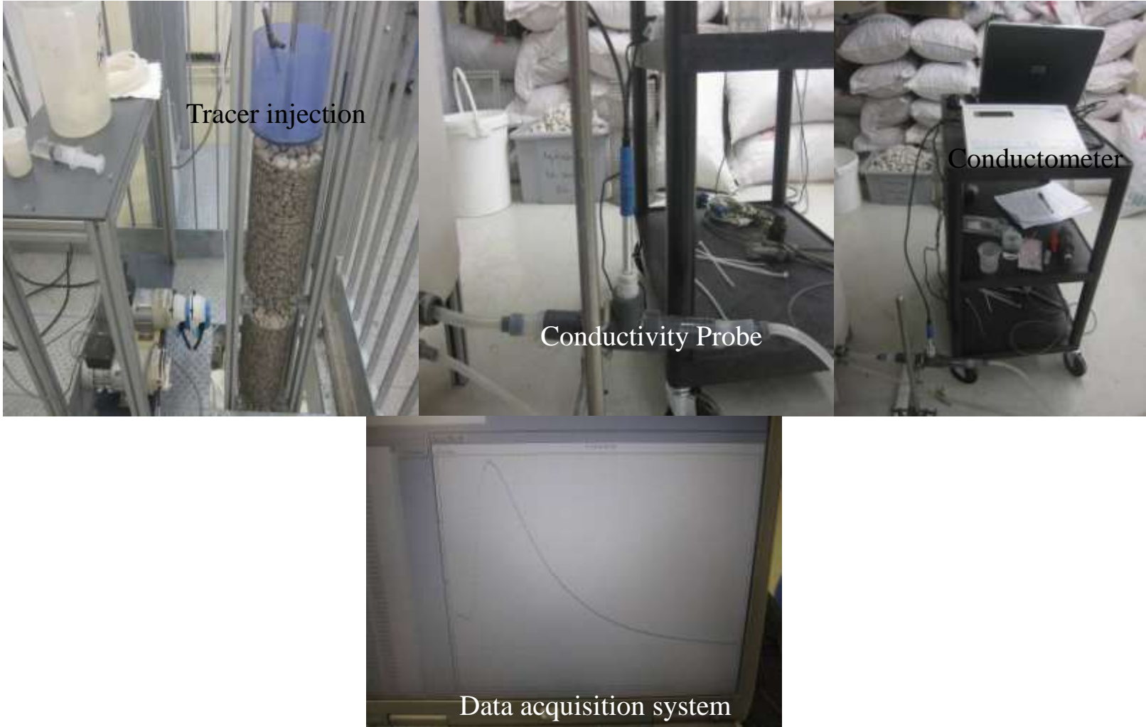
Figure A6-3: Experimental devices for RTD measurements
