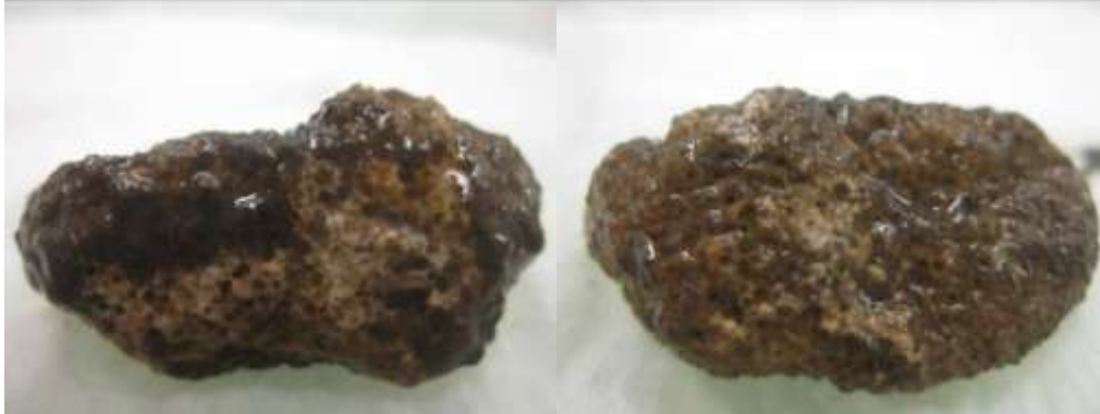
Figure A10-2: Medium particle coated with biofilm, in period 3 of biological experiments, high OLR, 1000 CODt input from real WW.
