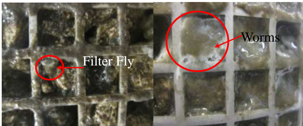
Figure A10-3: Photos of filter fly and worms observed in the packing bed and surface of biofilm during period 3, high OLR, real WW.
