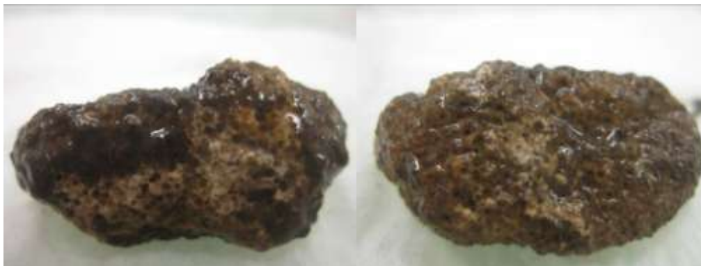
Figure A10-2: Medium particle coated with biofilm, in period 3 of biological experiments, high OLR, 1000 CODt input from real WW.
