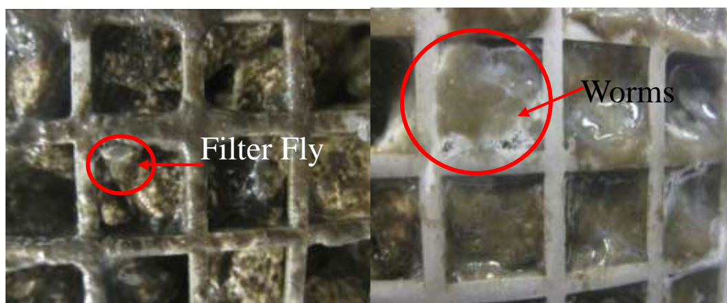
Figure A10-3: Photos of filter fly and worms observed in the packing bed and surface of biofilm during period 3, high OLR, real WW.
