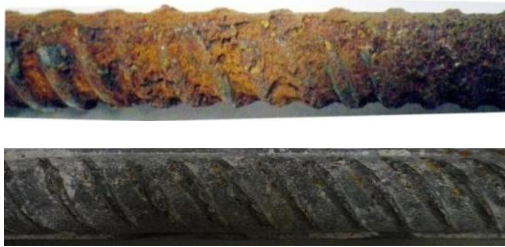
(a) Comparison of general corrosion
