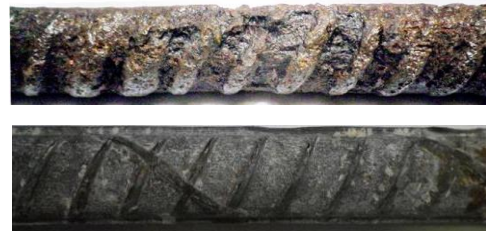
(b) Comparison of pitting corrosion
