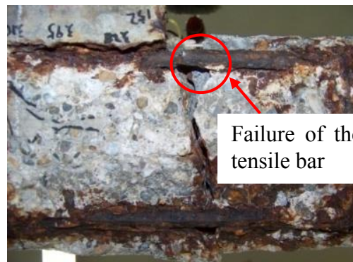
Figure 5-3 Experimental test on the corroded beam B2C13
