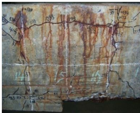
Figure 5-3 Experimental test on the corroded beam B2C13
