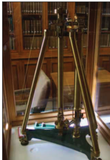
Fig. 2.2.3: Repsold's absolute pendulum used by Joaquín Barraquer y Rovira to realize the first absolute measurements of gravity in Spain (1982, National Astronomic Observatory of Madrid). Pendulum owned by The National Geographic Institute of Spain (IGN).
