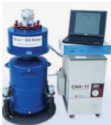
Fig. 2.2.8: New \bar{x} Grav superconducting gravimeter, manufactured by GWR Instruments (extracted from GWR website, http://www.gwrinstruments.com ).
