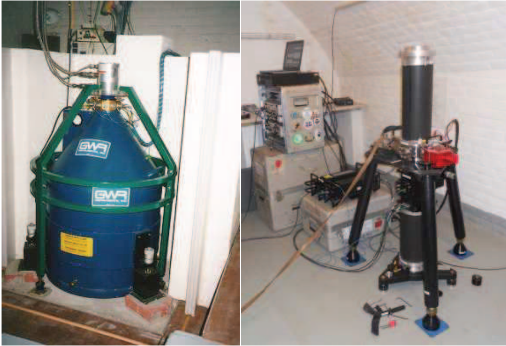
Fig. 4.22: Pictures of both, the superconducting gravimeter SG C026 (left) installed at the J9 Gravimetric Observatory of Strasbourg, and the absolute gravimeter FG5#206 (right), used in most of the calibration experiments carried out at J9 Observatory since 1996.
