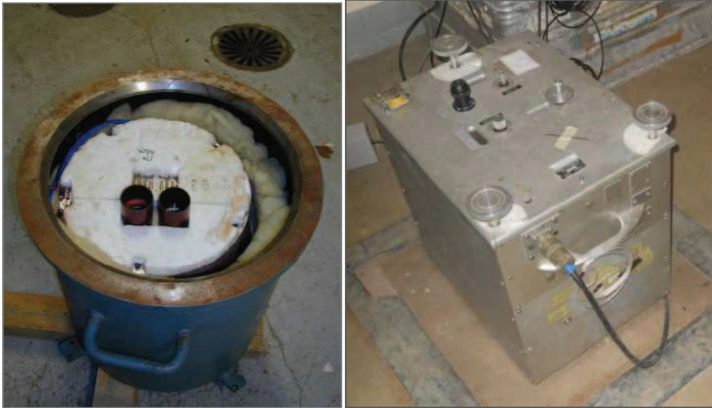
Fig 3.7: Pictures of the thermal insulated boxes where the spring gravimeters L&R ET005 (left picture) and the L&R ET11 (right picture) were installed at J9 Observatory.
