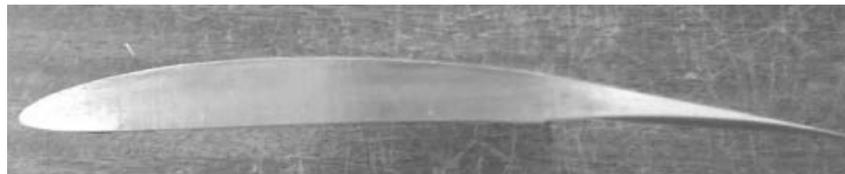
**Figure 1.14:** Turbine fan blade integrating an ABH extremity on the trailing edge (from [17])
