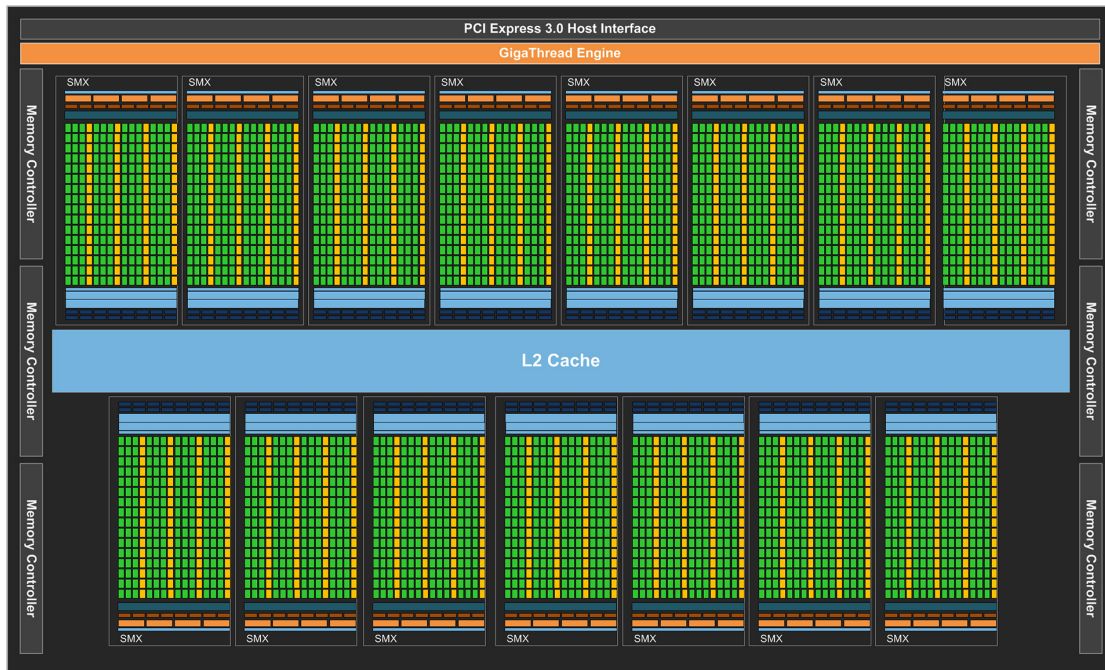
Figure 1.3 – Architecture of the NVIDIA Kepler GK110.
