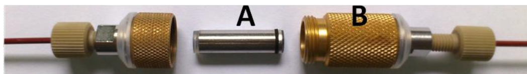
Figure 16. The support for silica particles with immobilised enzyme. A: cartridge, B: the cartridge nest.
