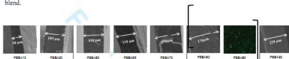
255 Fig. 2: SEM observations of cryofractured films after PEO extraction by water (PBSA 90 was 256 observed with a twice lower magnification) and CLSM microphotograph of PBSA80 showing 257 fluorescein-labeled PEO nodules embedded in PBSA matrix (scale: square size 75 \times 75 \mu\text{m}^2 ).
