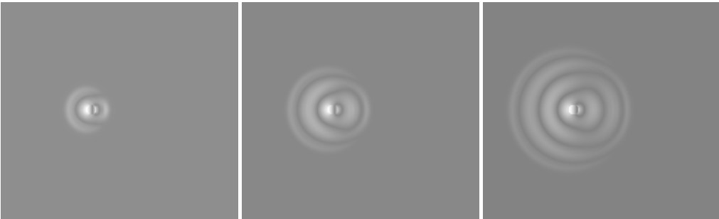
Figure 3.4: Instantaneous pressure magnitude of the scattered field p_s at three different times.
