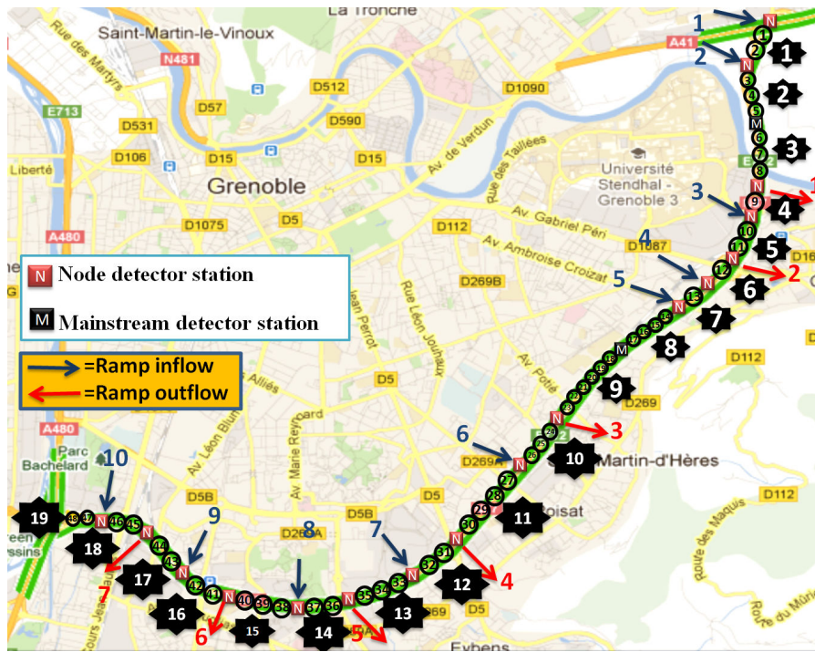
Figure 5.14: Freeway division considering discretization in cells.
