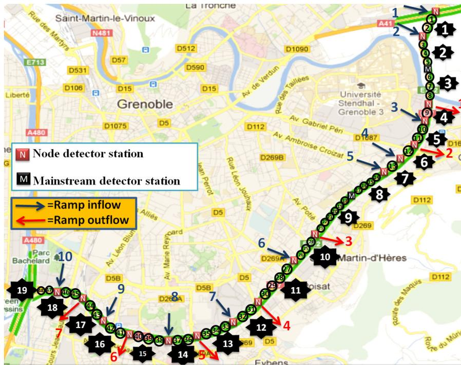
Figure 5.14: Freeway division considering discretization in cells.
