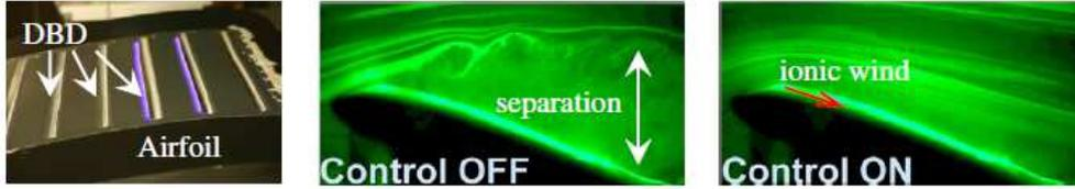
Figure 2.1.3: Flow reattachment using an array of DBD actuators [figure 9c from (Caruana (2010))].
