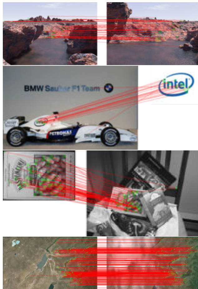
Figure 1.1: Examples of SIFT applications (excerpt of the IPOL demo archive).
