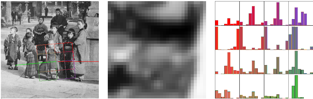
Figure 3.9: SIFT descriptor construction. No explicit re-sampling of the described normalized patch is performed. The normalized patch \mathcal{P}^{\text{descr}} is partitioned into a set of n_{\text{hist}} \times n_{\text{hist}} subpatches (default value n_{\text{hist}} = 4 ). Each sample (m,n) inside \mathcal{P}^{\text{descr}} , located at (m\delta^o, n\delta^o) , contributes by an amount that is a function of their normalized coordinates (\hat{x}_{m,n}, \hat{y}_{m,n}) (see (3.24)). Each sub-patch \mathcal{P}_{(i,j)}^{\text{descr}} is centered at (\hat{x}_i, \hat{y}_j) .
