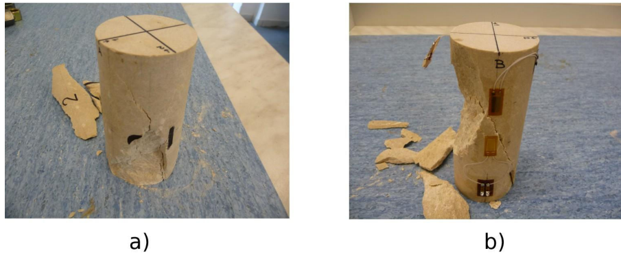
Figure 3.11: Failure mechanism for two specimens obtained within the experiment: a) the detachment of the material is noticed at the lower part of the specimen, b) the diagonal failure is pronounced
