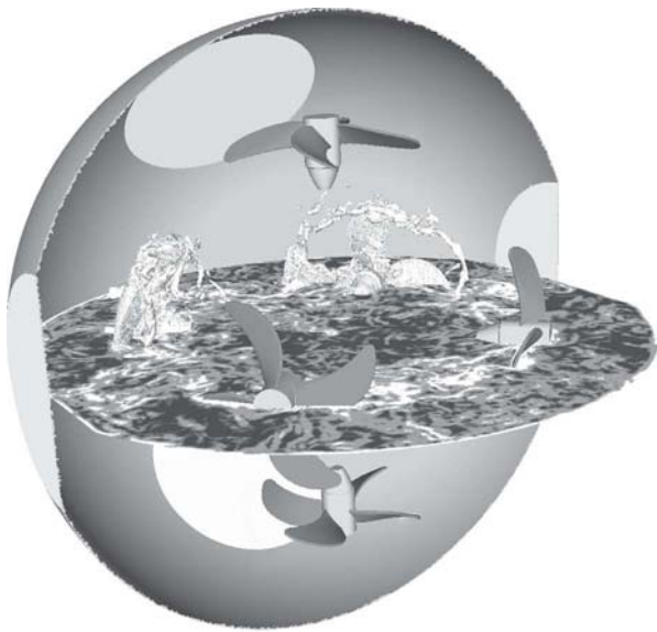
(a) Sketch of the geometry. |\nabla \vec{u}| instantaneous field in the central plane and iso-surfaces of vorticity in fan regions (for 2 fans only).
