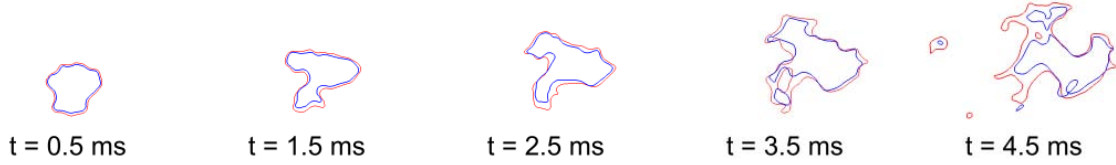
Figure 7.23: Flame propagation illustrated by instantaneous isolines of c^* = 0.9 . — : T_b^0 = T_{ad} = 2050 K ; — : T_b^0 = T_{ad} + 200 = 2250 K.
