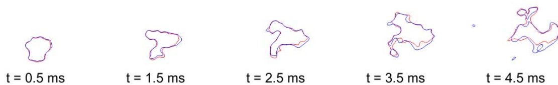
Figure 7.19: Flame propagation illustrated by instantaneous isolines at c^* = 0.9 . — : velocity field unchanged (Fig. 7.18(a)) ; — : velocity field set to zero (Fig. 7.18(b)).
