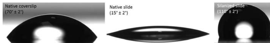
Figure 3.4 – Water in air static contact angle of (from left to right): native glass coverslip, native glass slide, silanized glass slide. The same static contact angle is found for silanized glass coverslip.
