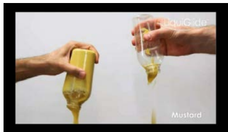
Figure 4.1 – Reproduction from LiquiGlide company. The left mustard pot does not exhibit slip at the walls whereas the right mustard pot does. The slippery pot is completely cleared out.
