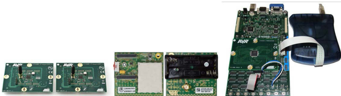
Figure 3-7 Photos of ATMEGA128RFA1 PCBA, ATMEGA128RFA1 Evaluation Kit and STK 600 with AVR JTAGICE mkII debugging tool
