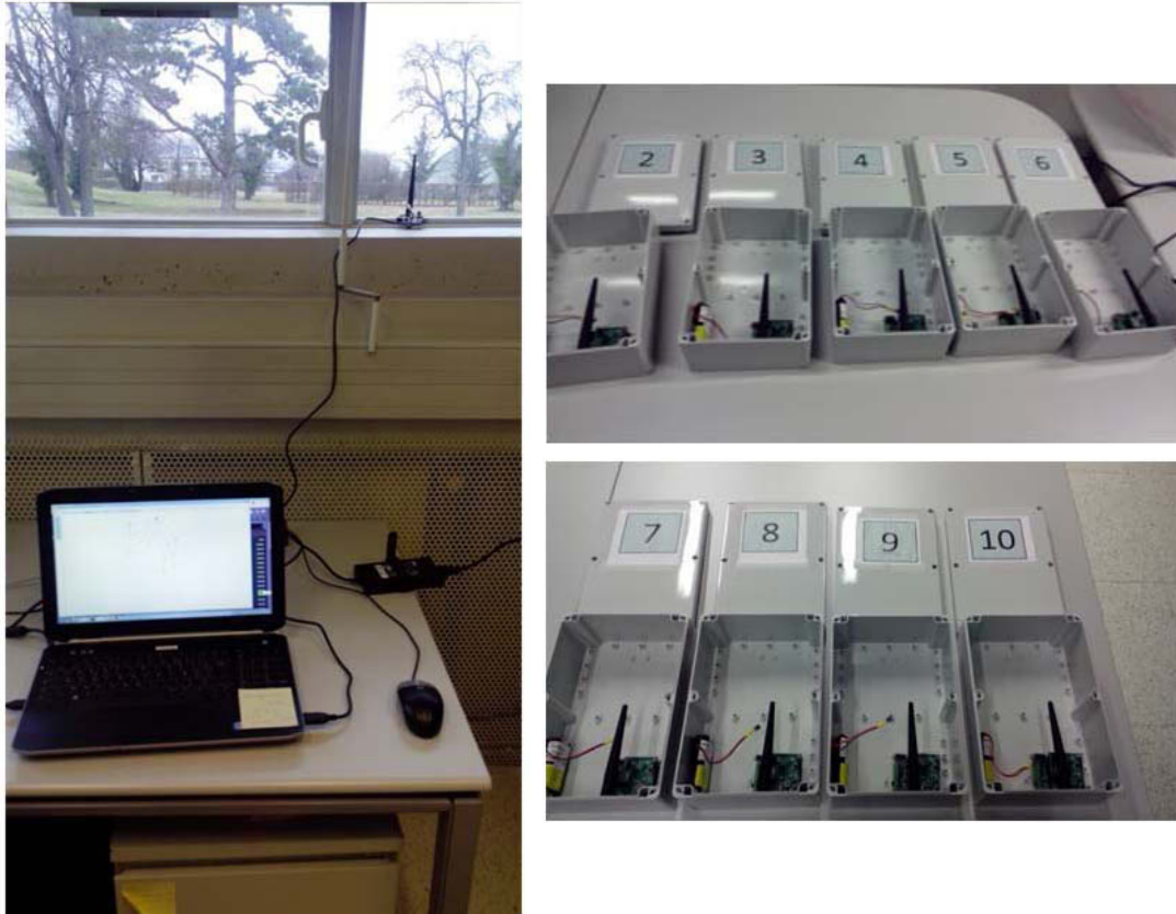
Figure 5-11 Testbed setup: sink node and 9 IWoTCore Ext_MiLive nodes for outdoor environment experiments
