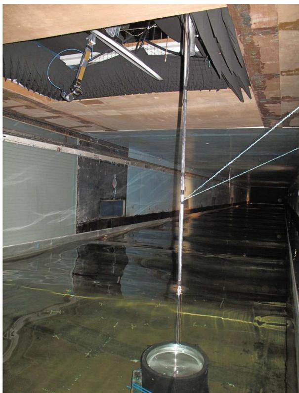
**Figure 2.** View of the wind tunnel, the parabolic antenna, the open waveguide, and the radar source fixed at the end of a sidearm adjusted in a crosswind azimuthal position. The whole radar system is mounted on two rotating plates set up above the tunnel roof opening and surrounded by radar absorbers. The wave gauges and the optical receiver of the slope measuring device immersed in water can be seen on the right side of the radar section.
