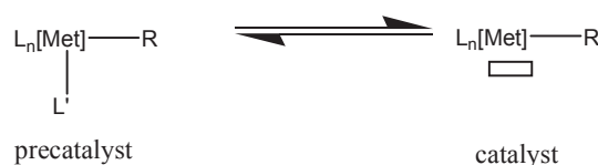
Figure 23. Schematic activation of a monocomponent catalyst, with R a carbon or H
