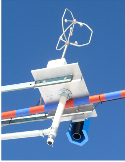
Fig. 4. Ultrasonic anemometer and snow-depth sensor (Jenoptik) (H.Bellot/Irstea).
