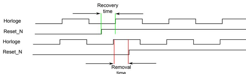
FIGURE 3.20 – Exemple de recovery time et removal time.
