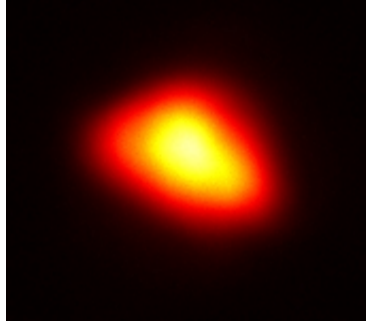
FIGURE 2.20 – Transverse profile of the laser pulse generating the bunch at PHIL for the measurement of Fig. 2.17. The image size is 171 * 151 pixel 2 and one pixel corresponds to 15.5 \mu\text{m} .
