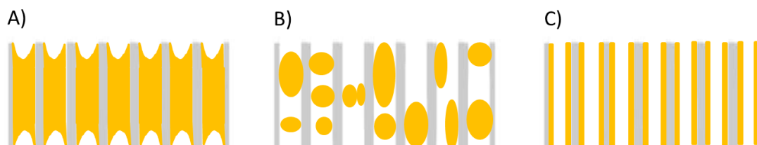
Figure 2.7: Possible scenarios which can describe the IL confinement in the AAO. a) Concave meniscus formation generated by the tension surface between the liquids and pores walls b) IL drops not interconnected between each others (or equivalently bubbles in the liquids). c) IL film formation on pores surface.
