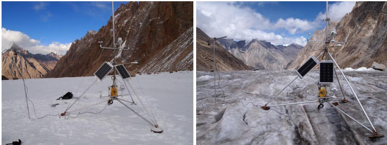
**Figure 5.3.** Photographs of AWS-G on Chhota Shigri Glacier taken on 09 October 2012 (left panel) and on 22 August 2013 (right panel) (copyright: Mohd. Farooq Azam). SR50A mounted on a separate pole drilled into the ice, is visible to the left of AWS-G.
