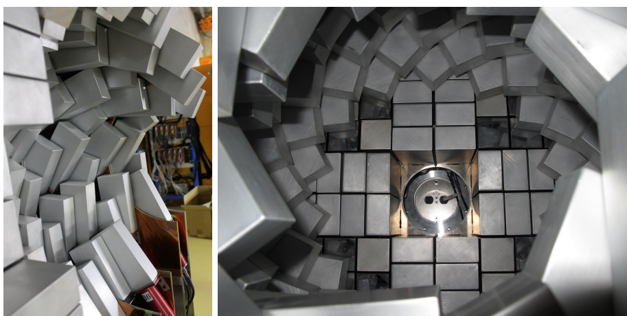
Fig. 4.4 – Picture of the DALI2 gamma array. (Left) Half of the DALI2 crystals, seen from downstream, with the first layer crystals clearly visible. (Right) DALI2 crystals geometry shown from upstream. The last 11 th layer of crystals is shown in the background.
