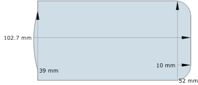
Fig. 5.16 – Scheme of the \text{LH}_2 target of 102.7(10) mm when cooled down and filled with hydrogen.
