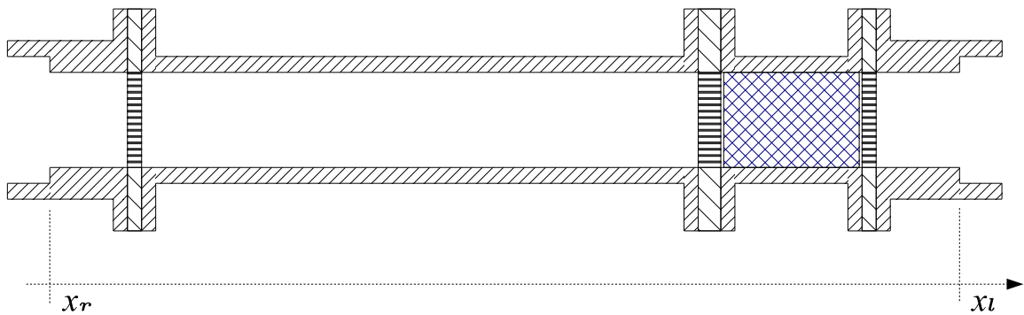
Figure 3.10: Sketch of the inverted ThermoAcoustic Core.
