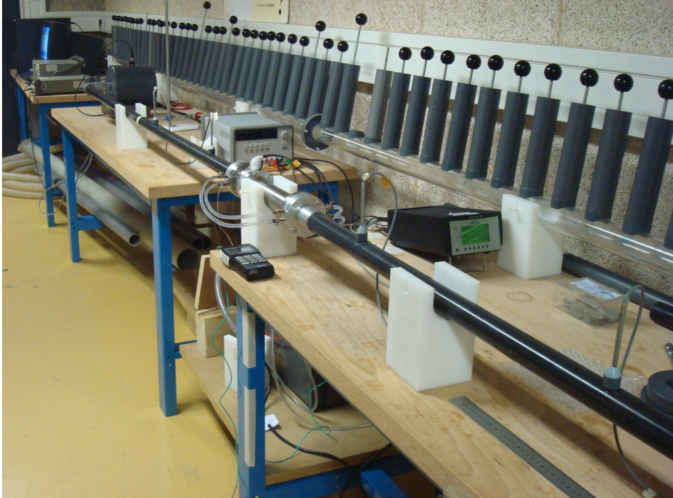
Figure 3.4: Experimental setup - Two-Load Method.
