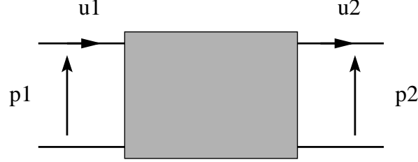
Figure 2.2: Adopted pressure-volume velocity convention for the quadrupole description; anti-symmetric orientation.
