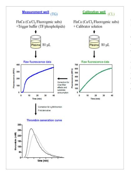
Figure 2.1. Diagram of the CAT method measures for a plasma sample.
