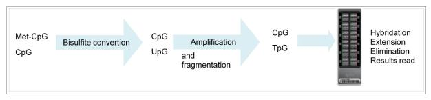
Figure 7.3. Methylation determination protocol.
