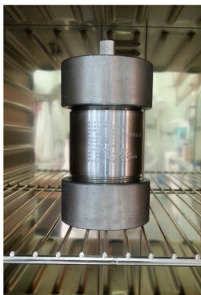
Figure 3.1: Hydrothermal reactor used for \text{TiO}_2 nanopartciles preparation.
