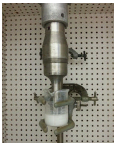
Figure 3.2: Ultrasonic horn to prepare \text{TiO}_2 and ZnO paste
