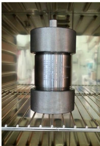
Figure 3.1: Hydrothermal reactor used for TiO<sub>2</sub> nanoparticles preparation.
