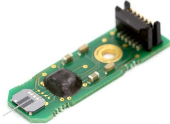
Figure D.1 – FemtoTools force sensor. It measures down to tens of nN with a capacitive deflection technology.
