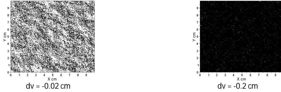
Figure 3-20 continuation Contact points between surface S1 and its corresponding DEM surface as a function of their vertical relative distance dv . The black points denote contact between both surfaces.
