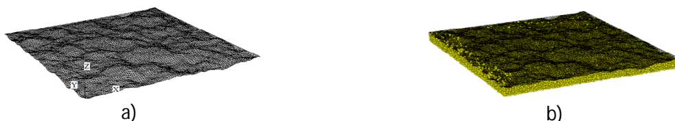
Figure 3-18 a) mesh of the synthetic surface used to generate the DEM joint, b) synthetic mesh and DEM joint generated, c) resultant DEM joint, d) regular grid to obtain the height of the DEM surface, e) elevation map of the synthetic surfaces used as a mold, f) elevation map of the DEM surface.
