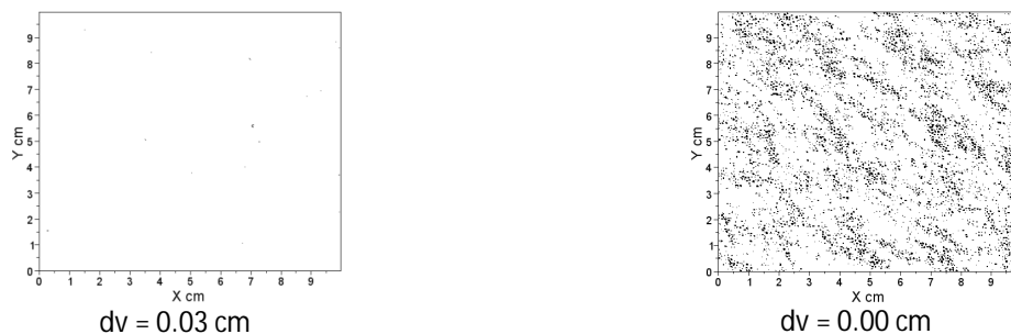
Figure 3-20 Contact points between surface S1 and its corresponding DEM surface as a function of their vertical relative distance dv . The black points denote contact between both surfaces.
