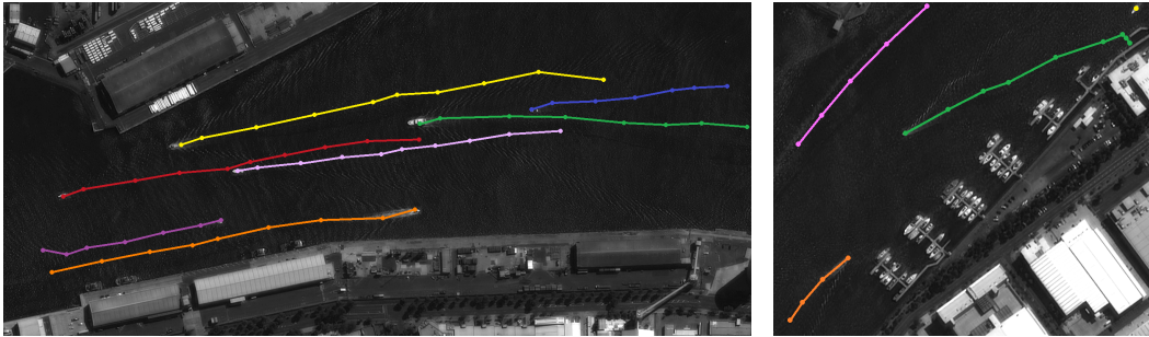
Figure 5.13: Detection and tracking results on two sequences of real satellite images taken at different angles (©INRIA). Each color represents a different track. Left: Tracking results on the first image sequence up to frame 10. Right: Tracking results up to frame 13 of the second image sequence.
