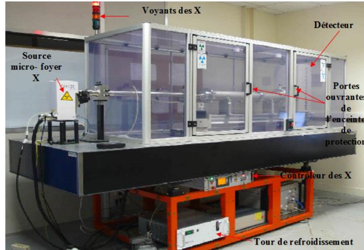
Figure II.12: Montage SAXS utilisé
