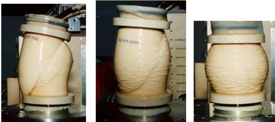
Figure 2.34: Three specimens of Hostun sand loaded to failure at \sigma_3=400\text{kPa} in drained condition. From left to right: dense, medium dense, loose (from Desrues (2004))
