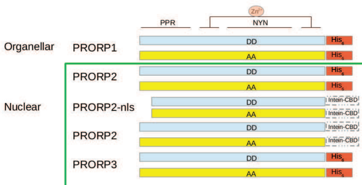
Figure 3.2: Scheme of PRORP constructs used during my work: -nls without nuclear localization signal, DD - wild type with conserved aspartates in active site, AA - double catalytic mutant with aspartates mutated into alanines, NYN - catalytic domain, PPR - pentatricopeptide repeat, Zn - bipartite zinc binding domain, intein-CBD - cleaved chitin binding domain during purification.
