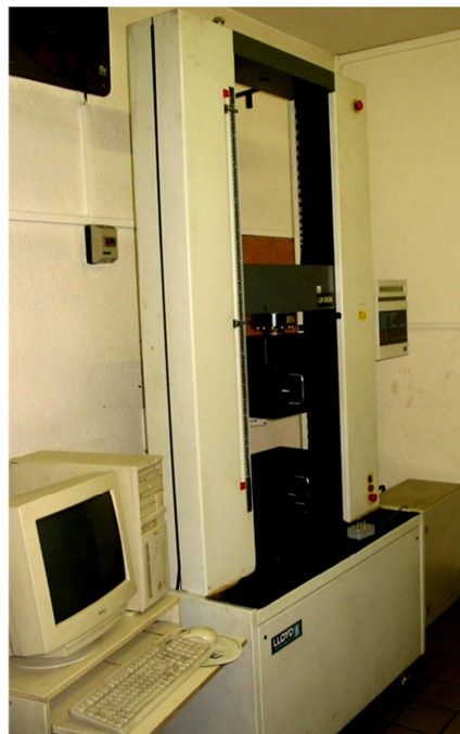
Figure 4.61. Machine de traction de COBRA.
