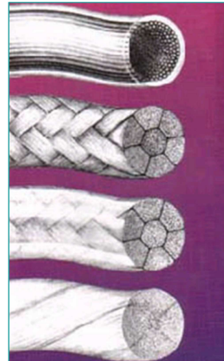
Figure A.13. Fils multi-filaments.
