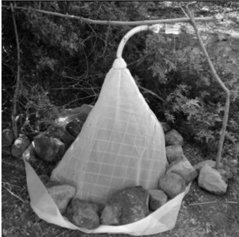
SD 1: Modified soil emergence traps used to record the emergence of adults from the soil
