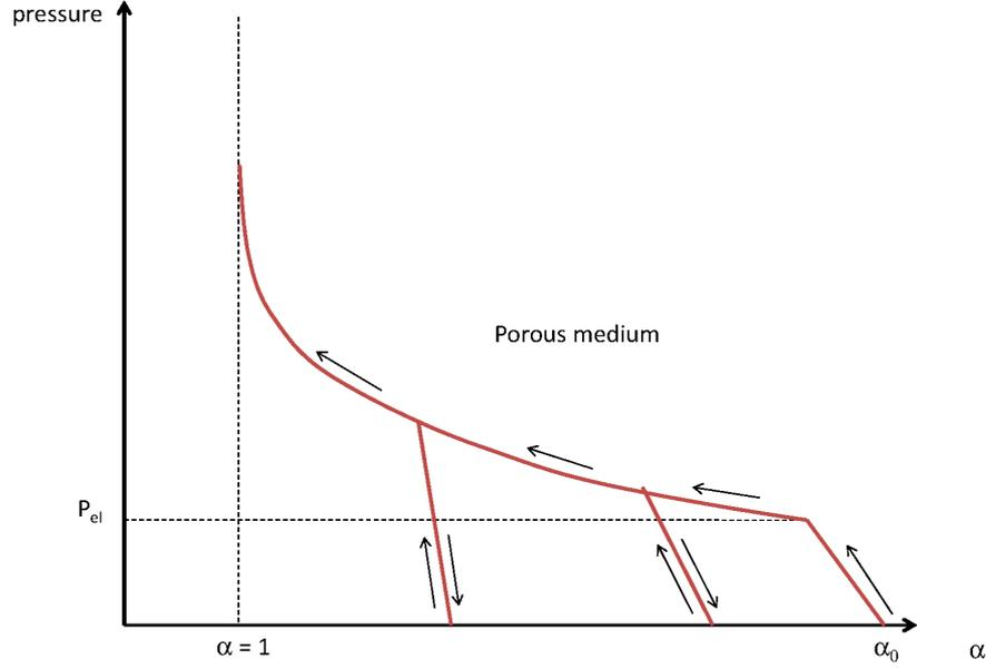
Figure 3.5: The  $P - \alpha$  model.  $P$  is the pressure of the grain-water mixture.  $\alpha$  is the ratio of this mixture phase over all the phases. When  $\alpha = 1$ , no air remains in the medium: the soil is fully compacted. For  $\alpha > 1$ , some porosity exists inside the medium.
