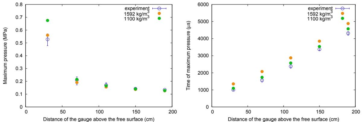
Figure 5.60: Same as figure 5.59 but for DOB of 8 cm. Except for the first peak, all the pressures provided close results compared to the experiments. Moreover with an initial density of  $1100 \text{ kg.m}^{-3}$ , all the time results were almost in the range of the experiments.
