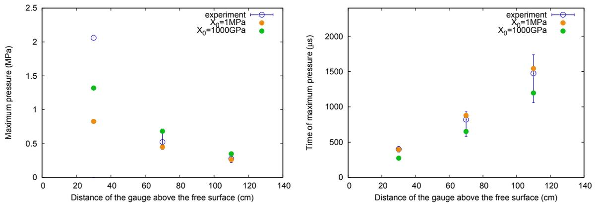
Figure 5.69: Maximum pressures (left) and their respective times (right) for a DOB of 3 cm in experiments, in simulations with  $X_0 = 1 \text{ MPa}$  and 1000 GPa. Compared to the experiments, the maximum pressures are too large, except for the first peak which is closer. The times of the maximum pressures are a little too short.
