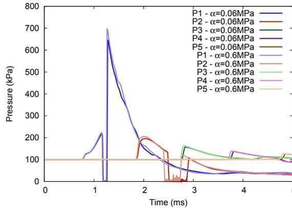
Figure 5.64: Comparison of the pressure profiles at the five outputs for a charge buried at 8 cm for two values of the initial shear stress  $\alpha$  (60 and 600 kPa). When the yield surface widens, the pressure signals arrive a little earlier and the pressure peaks are a little increased.
