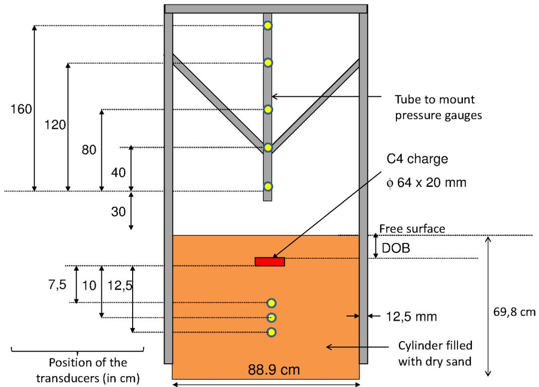
Figure 5.5: Small scale experimental setup of Bergeron et al. (1998) and position of the pressure transducers. Dry sand was used.
