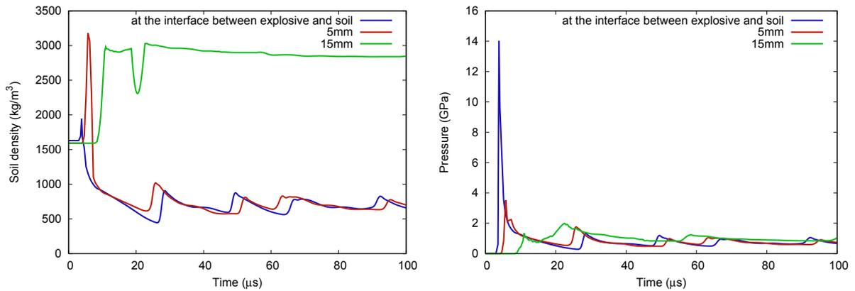
Figure 4.36: Time course of the density (left) and of the pressure (right) in the soil in three fixed points (at the interface with the explosive, at 5 mm and 15 mm from the interface in the soil). Our model is used for the soil.
