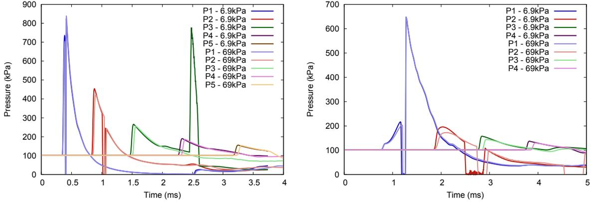
Figure 5.67: Comparison of the pressure profiles at the five outputs for charges buried at 3 cm (left) and at 8 cm (right) for  $T = 6.9\text{kPa}$  and  $69\text{kPa}$ . With  $T=69\text{kPa}$ , the pressure waves are delayed and the pressure peaks are smaller, which is strange since the soil is more elastic.
