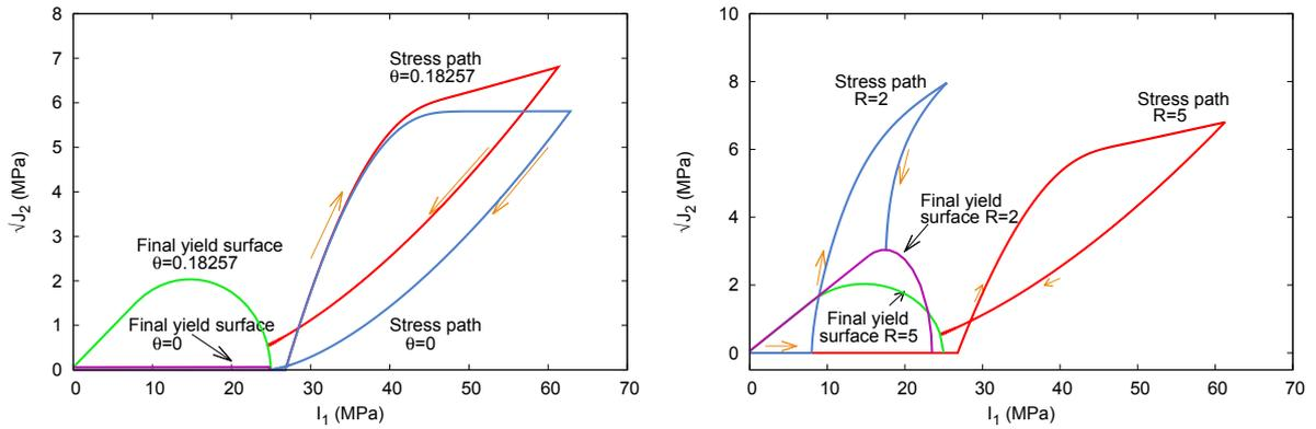
Figure 2.9: On the left, comparison of the stress paths obtained for  $\theta = 0$  and for  $\theta = 0.18257$ . On the right, comparison of the stress paths obtained for  $R = 2$  and  $R = 5$ . Both parameters change the shape of the yield surface which has a direct influence on the direction of the stress path.
