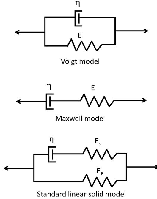
Figure 2.1: Three models of linear viscoelasticity. They are constituted by springs and dashpots. Dashpots have a coefficient of viscosity  $\eta$ , and thus an intrinsic time to react, whereas the deformation obtained with the spring and its stiffness  $E$  is instantaneous.
