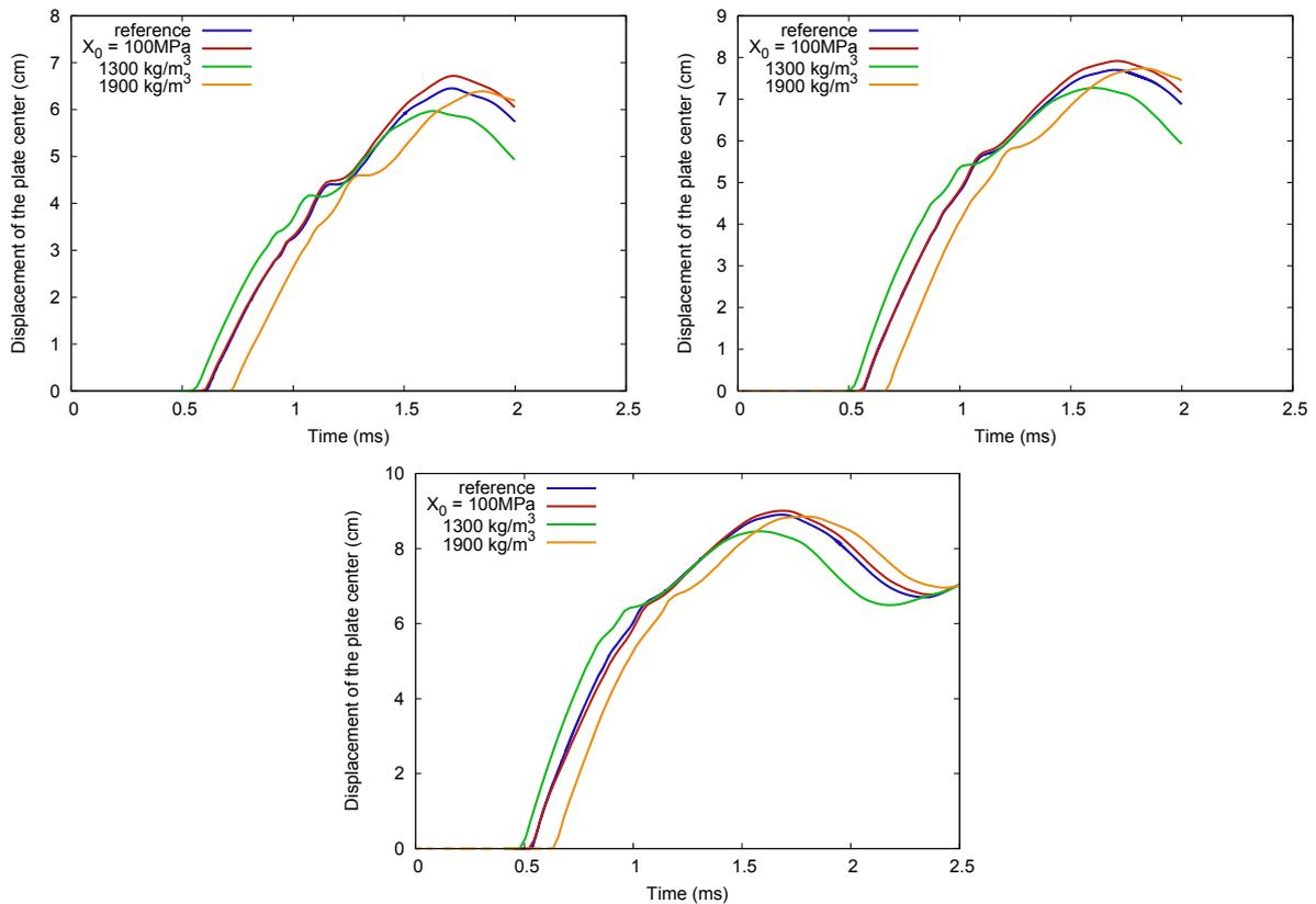
Figure 6.13: Time course of the vertical displacement of the central point of the plate for 6 kg (top left), 8 kg (top right) and 10 kg (bottom) of TNT. The reference curve corresponds to the simulation with the parameters detailed in table 2.1. The other curves differ each by a parameter.
