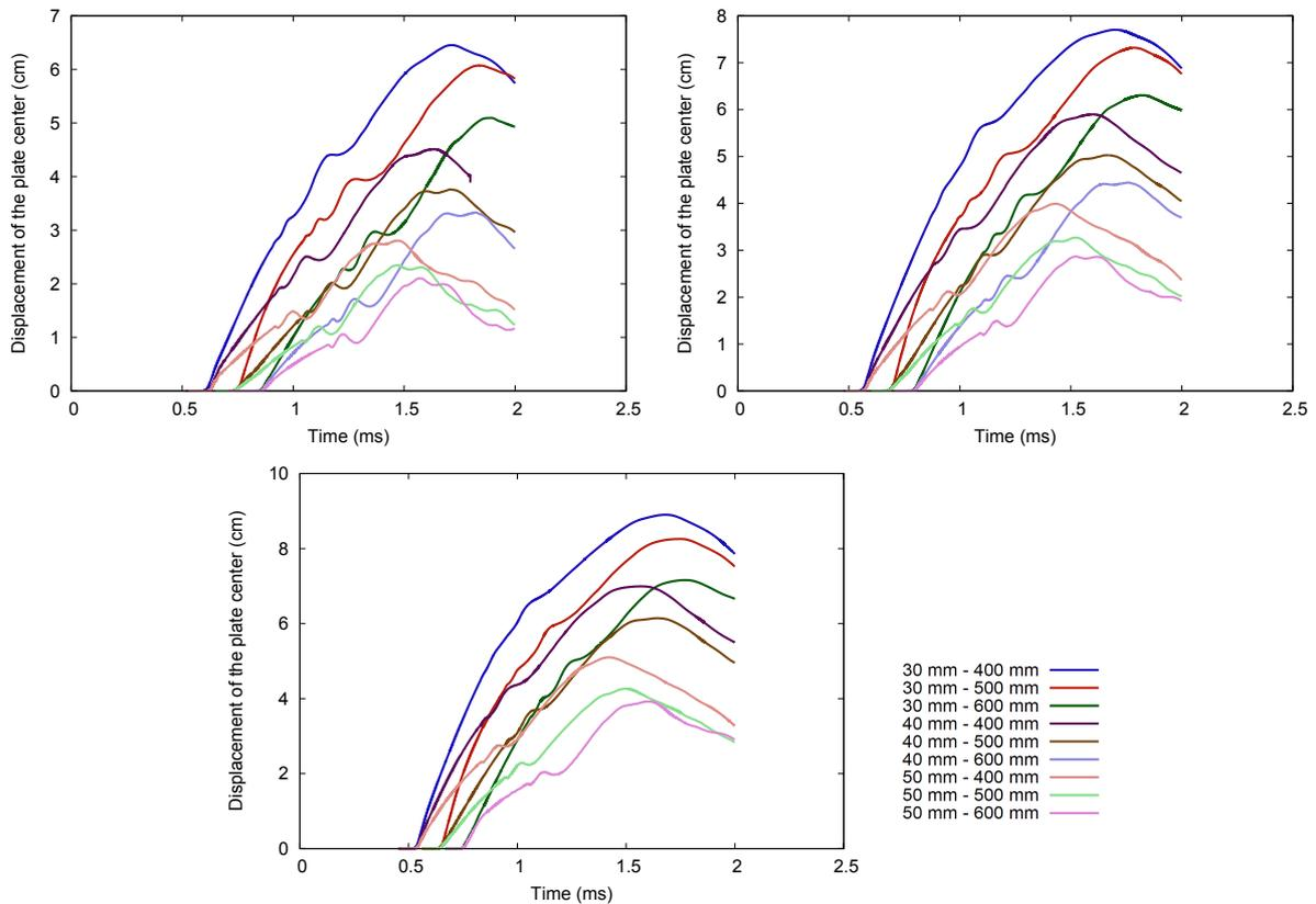
Figure 6.12: Time course of the vertical displacement of the central point of the plate for 6 kg (top left), 8 kg (top right) and 10 kg (bottom) of TNT. Three thicknesses of plate (30, 40 and 50 mm) and three stand off distances were tested (400, 500 and 600 mm).
