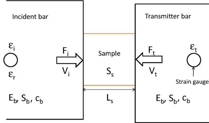
Figure 4.4: Parameters of the bars and the sample used to derive the strain rate in the specimen.
