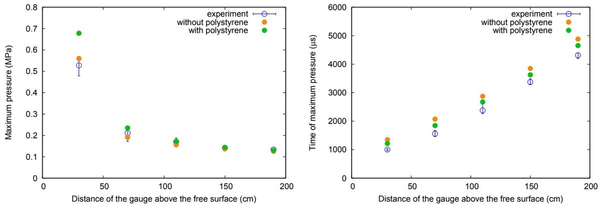
Figure 5.47: Maximum pressures (left) and their respective times (right) for a DOB of 8 cm in experiments, in simulations with and without representing the polystyrene surrounding the explosive. The simulations are closer to the experiments when the polystyrene is taken into account.
