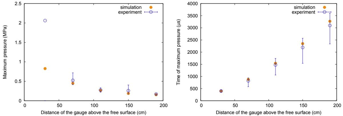
Figure 5.42: Maximum pressures (left) and their respective times (right) at the five outputs for a DOB of 3 cm. Apart from the first output where a huge pressure difference exists between the experiments and the simulations, all the other simulation outputs fit with the experiments.
