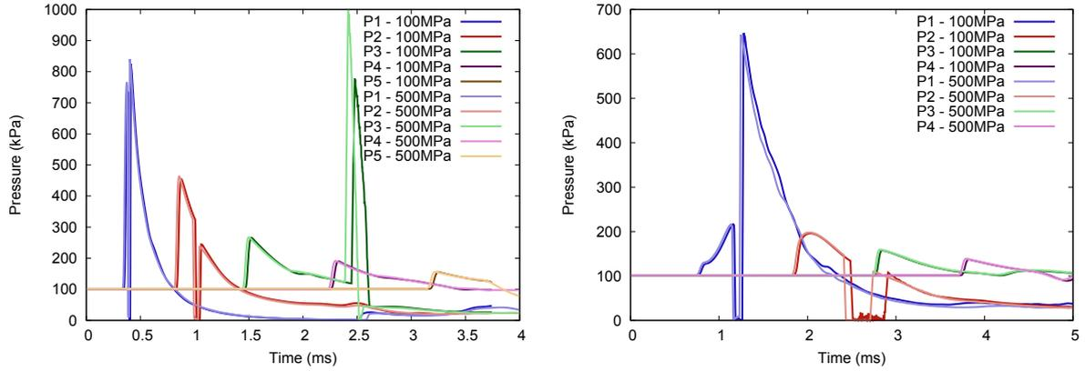
Figure 5.55: Time profiles of the pressures at the five outputs for charges buried at 3 cm (left) and 8 cm (right) for  $K_0 = 100$  and 500 MPa. With an initial bulk modulus of 500 MPa, the waves arrive a little earlier, but the peaks are very close for the two elastic moduli.
