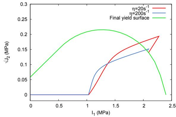
Figure 2.13: Comparison of the stress paths obtained for  $\eta = 20$  and  $\eta = 200 \text{ s}^{-1}$  with a strain rate of  $10 \text{ s}^{-1}$ . The effects of  $\eta$  are the contrary of those observed for  $f_0$ : the smaller the value of  $\eta$ , the more viscoplastic and thus elastic the behavior of the material is.
