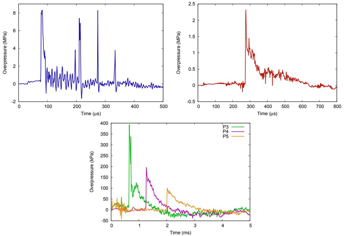
Figure 5.17: Time course of the pressure for the first (top left), second (top right), third, fourth and fifth gauges (bottom) of the first shot.
