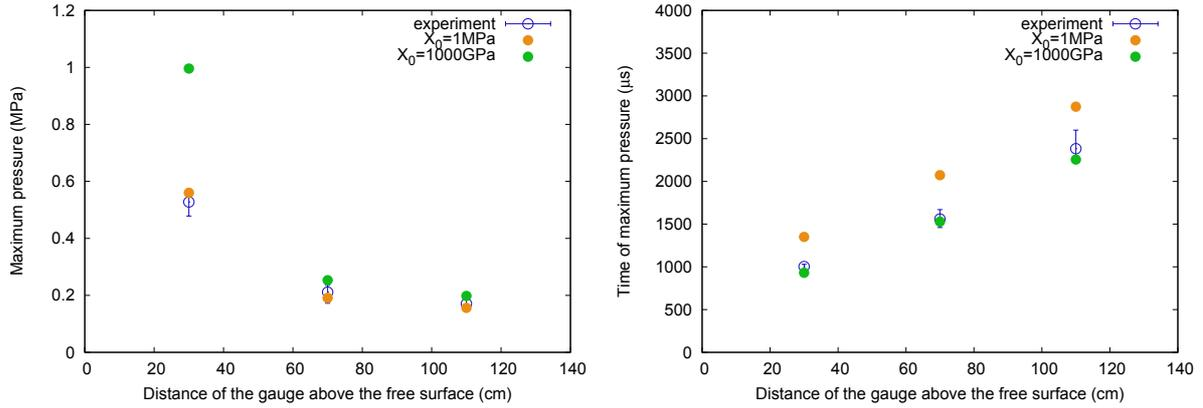
Figure 5.70: Same as figure 5.69 but for a DOB of 8 cm. Like for the depth of burial of 3 cm, the maximum pressures are too large compared to the experiments. As for the times of arrival, an increase of  $X_0$  seems appropriate since the time of the maximum pressure has decreased a lot. The time shift between experiments and simulations does not exist anymore.
