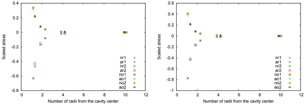
Figure 4.24: Static value of radial and orthoradial stresses at various radii from the cavity center with a mesh size of 10 mm (left) and 5 mm (right). The stresses have been scaled with the initial pressure (10MPa). (n: numerical solution; a: analytical solution; r: peak of the radial stress; o: peak of the orthoradial stress; 1: equatorial plane; 2: radial plane)
