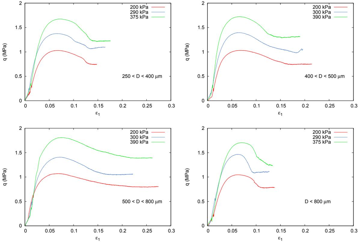
Figure 1.7: Curves relating the deviatoric stresses to the axial strain with uniform grain sizes  $D$  ( $250 < D < 400 \mu\text{m}$  (top left),  $400 < D < 500 \mu\text{m}$  (top right) and  $500 < D < 800 \mu\text{m}$  (bottom left)), and another sample (bottom right) with grain sizes smaller than  $800 \mu\text{m}$  (with a grain size repartition representative to the STANAG soil)
