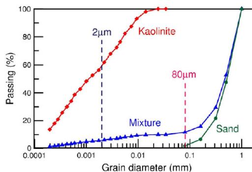
Figure 1.2: Particle size distribution of soil specimen used by Arlery et al. (2010) for plate impact experiments detailed in chapter 4.
