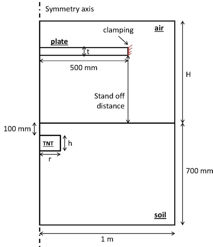
Figure 6.9: Extent of the mesh for the simulations of large quantity of buried TNT (6, 8, and 10 kg) to study its effect on a plate. The explosive has a radius  $r$  and a height  $h$ . The plate has a thickness  $t$ , a radius of 500 mm, and is located at a distance called stand off distance from the free surface of the soil. The extremity of the plate is clamped, allowing no displacement nor rotation. The height  $H$  of the mesh is chosen according to the stand off distance.
