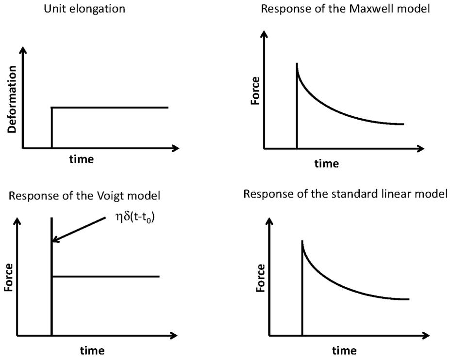
Figure 2.3: Relaxation function obtained for the three viscoelastic models submitted to a unit elongation.
