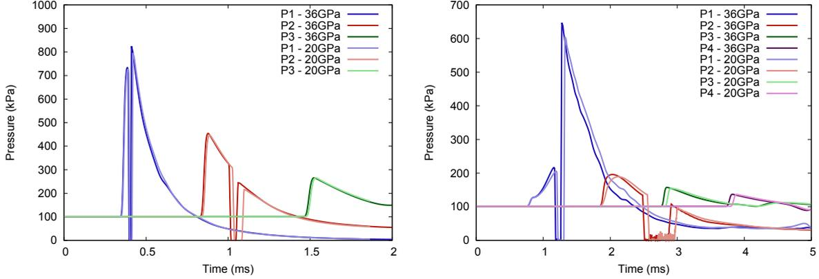
Figure 5.56: Comparison of the pressure profiles at the five outputs for charges buried at 3 cm (left) and 8 cm (right) for  $K_{wg} = 20$  and 36 GPa. With a bulk modulus  $K_{wg}$  equal to 20 GPa, the pressure waves are slightly delayed.
