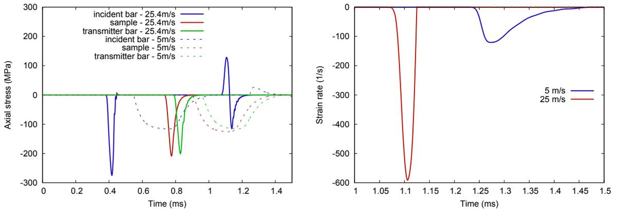
Figure 4.13: On the left, time history of the stresses in the bars and in the sample for two impact velocities (5 and 25.4 m/s). On the right, time history of the strain rate in the sample for two impact velocities (5 and 25.4 m/s).
