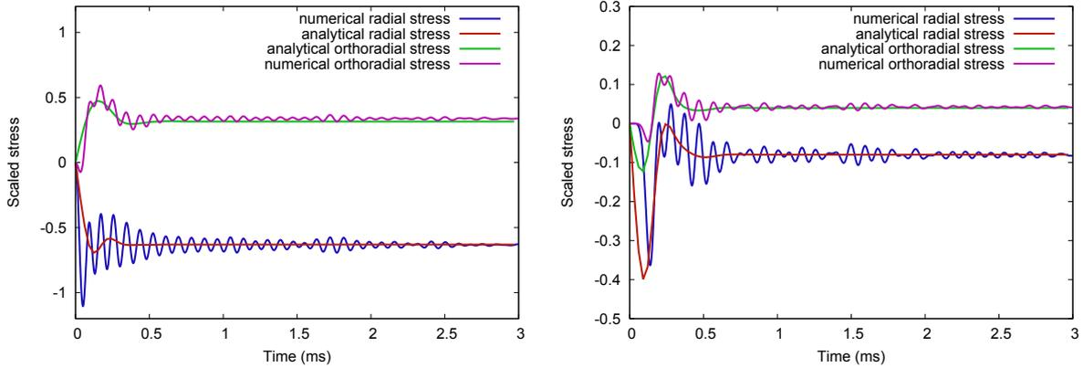
Figure 4.25: Analytical and numerical results of the radial and orthoradial stresses at 3 radii (left) and 9 radii (right) from the center of the cavity (element on the equatorial plane). The stresses have been scaled with the initial pressure (10MPa).
