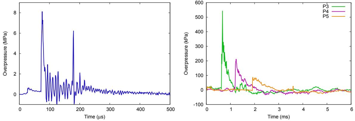
Figure 5.18: Time course of the pressure for the first (left), third, fourth and fifth gauges (right) of the second shot. A gravel may have hit the first gauge, provoking the peak which can be seen at around  $180 \mu\text{s}$ .
