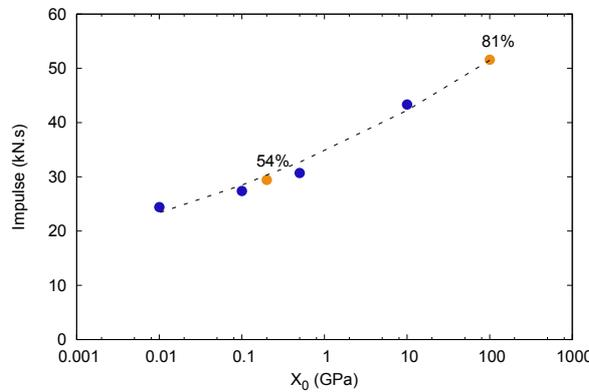
Figure 6.33: Influence of the initial value of the cap limit  $X_0$  on impulse. For  $X_0=200$  MPa and 100 GPa, the impulses are very close to those obtained in experiments for shots 6 and 4 respectively. The only difference between these two shots was the degree of saturation of the soil. For shot 4, it was equal to 81% whereas it was equal to 54% for shot 6. If all the other parameters are fixed, the initial value of the cap  $X_0$  can be linked to the degree of saturation of the soil.
