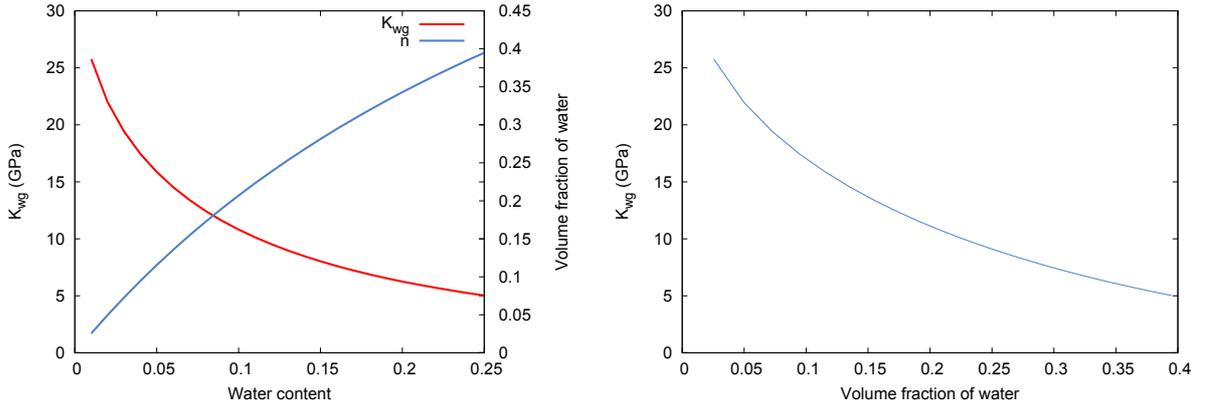
Figure 3.7: On the left, bulk modulus of the grain-water mixture  $K_{wg}$  and volumetric fraction  $n_w^\infty$  in relation to the water content  $w$ . On the right, grain-water mixture  $K_{wg}$  in relation to volumetric fraction  $n_w^\infty$ . A density of  $2610 \text{ kg.m}^{-3}$  was used for the density of the grains.
