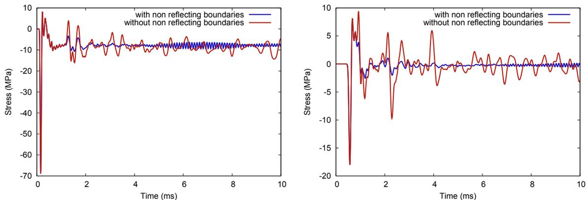
Figure 4.32: Time history of the radial stresses at 100 mm from the explosive or 4 radii from the detonation point (left), and 250 mm from the explosive or 10 radii from the detonation point (right). Simulations are run with fixed boundary conditions (so reflections can occur), and with transmitting boundaries (reflections are prevented).
