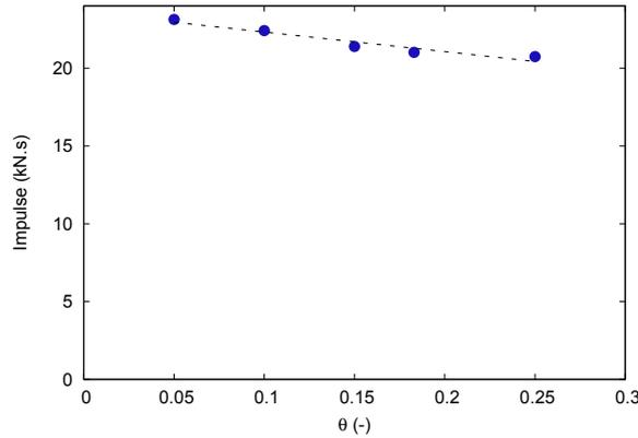
Figure 6.32: Influence of the value of  $\theta$  on impulse. The slope  $\theta$  and the friction angle  $\phi$  are related in the following way:  $\theta = (2/\sqrt{3}) \times \sin \phi / (3 - \sin \phi)$  or in inverse form  $\sin \phi = 3\sqrt{3}\theta / (2 + \sqrt{3}\theta)$
