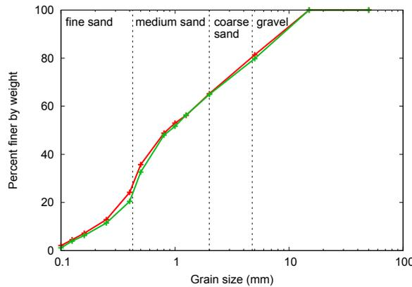
Figure 1.3: Particle size distribution of STANAG soil, obtained from ten sieves, with size holes from 100  $\mu\text{m}$  up to 5 mm. The two curves correspond to a grain size analysis obtained from two separate tests.
