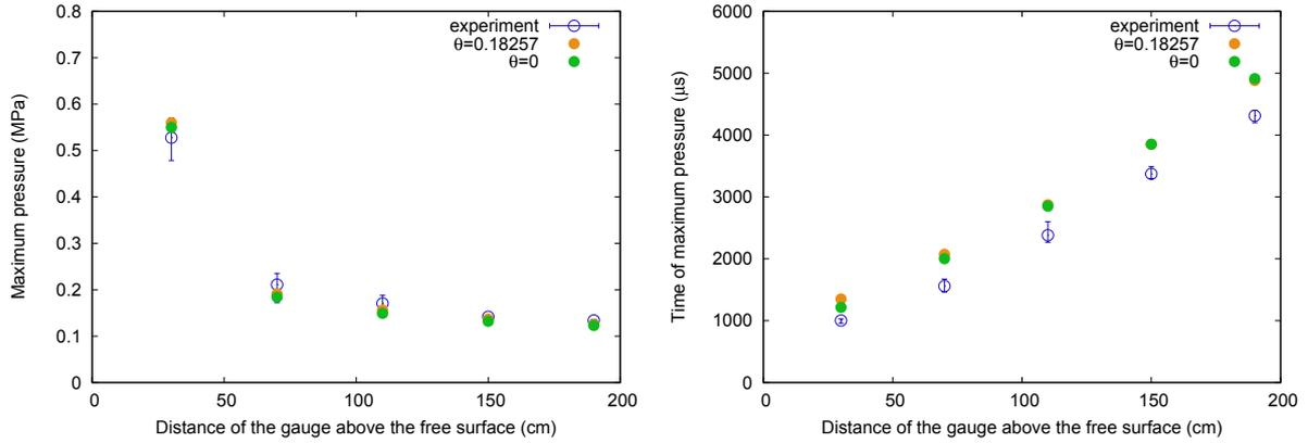
Figure 5.65: Maximum pressures (left) and their respective times (right) at the five outputs for a DOB of 8 cm in experiments, and in simulations with  $\theta = 0$  and  $\theta = 0.18257$ . With  $\theta = 0$ , the first pressure peak and its first time of arrival are closer to the experiments. Far away, there is no longer differences between the two values of  $\theta$ .
