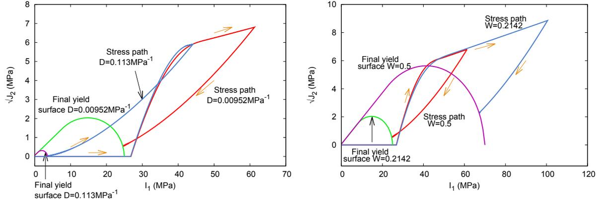
Figure 2.11: On the left, the stress paths obtained for  $D = 0.00952$  and  $0.113 \text{ MPa}^{-1}$  are compared. The larger the value of  $D$  is, the slower the displacement of the cap is. With  $D = 0.113 \text{ MPa}^{-1}$ , the cap hardens so slowly that during the relaxation step the stress path ends its way almost on the hydrostatic axis. On the right, comparison of the stress paths obtained for  $W = 0.2142$  and  $W = 0.5$ . The smaller the value of  $W$  is, the more the cap hardens.
