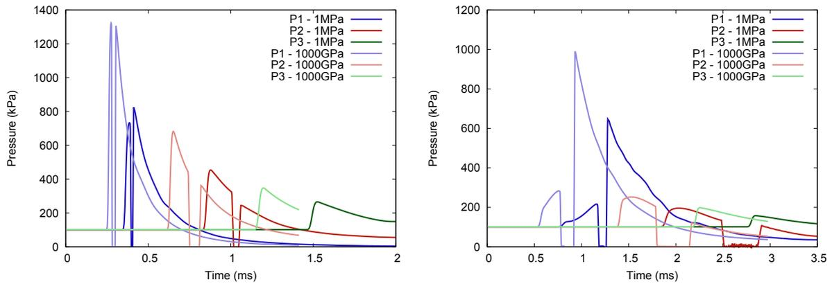
Figure 5.68: Comparison of the pressure profiles at the five outputs for charges buried at 3 cm (left) and 8 cm (right) for  $X_0 = 1 \text{ MPa}$  and 1 000 GPa. With a larger cap (so a wider yield surface), the pressure waves arrive much earlier and the pressure peaks are much larger.
