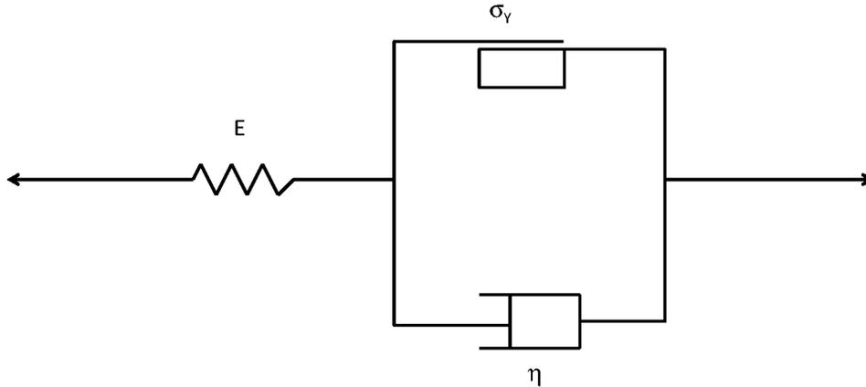
Figure 2.4: Rheological model for a viscoplastic material.
