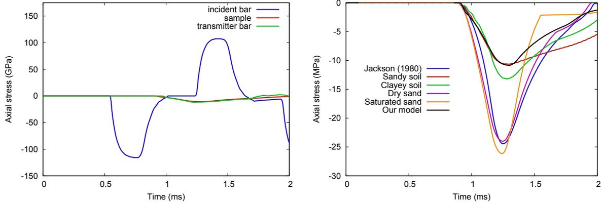
Figure 4.16: On the left, time history of stresses in the bars and in the sample modeled with our viscoplastic cap law. On the right, time history of stresses in the sample for various sets of parameters with the geologic cap model of LS Dyna and with our model.
