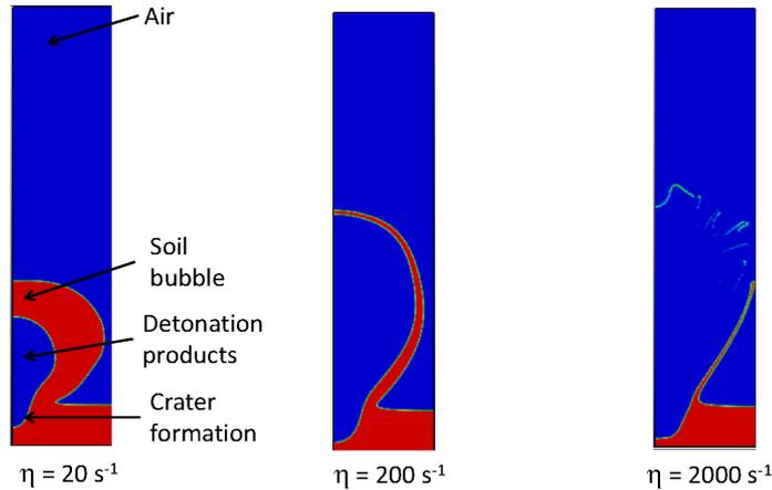
Figure 5.53: Contours of the volume fraction of soil for a depth of burial of 3 cm, for  $\eta = 20, 200$  and  $2000$  s<sup>-1</sup> at  $t = 2$  ms. The red color denotes the presence of the soil and the blue color the air.
