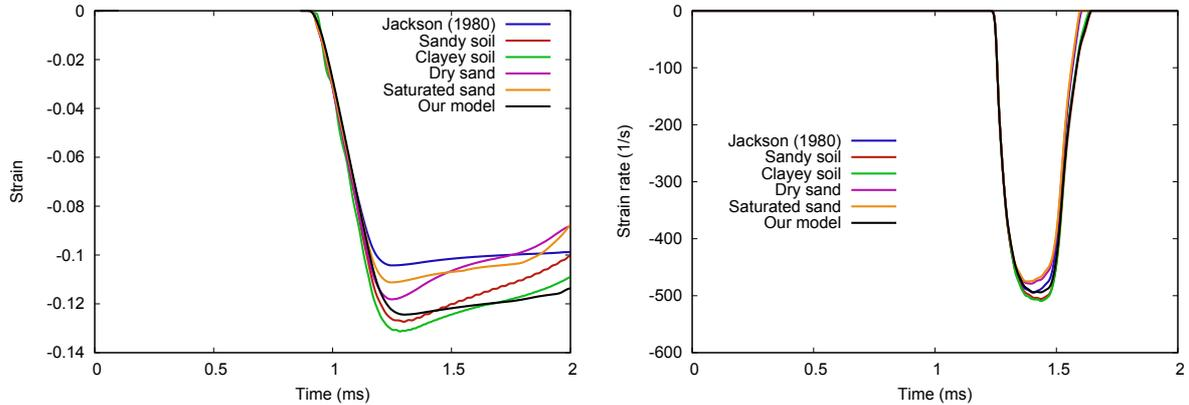
Figure 4.17: On the left, time history of strains in the sample for various sets of parameters with the geologic cap model of LS Dyna and with our model. On the right, time history of strain rates in the sample for various sets of parameters with the geologic cap model of LS Dyna and with our model.
