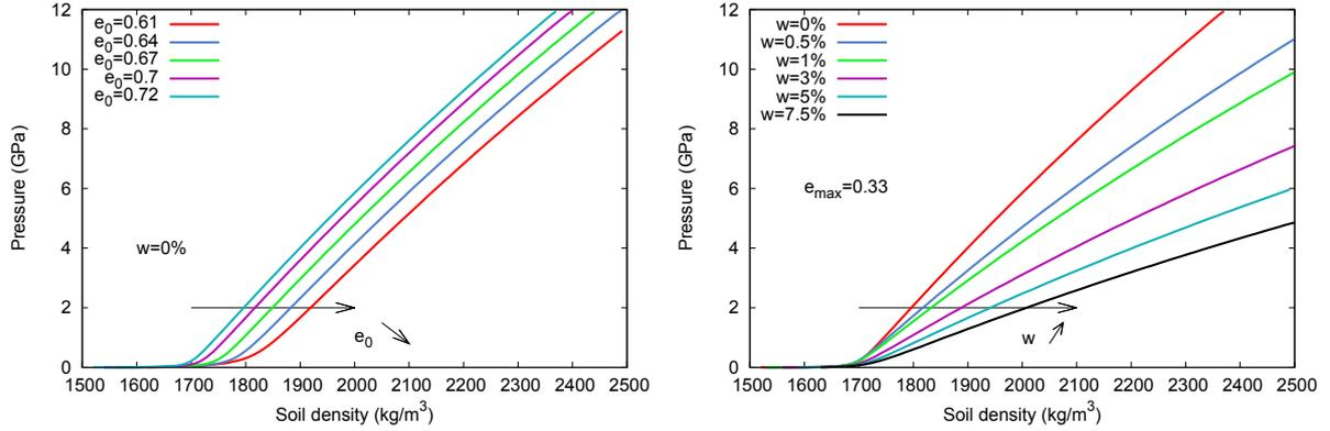
Figure 3.9: Pressure-density curves for dry loose sandy gravel with various initial void ratios (left) and with a maximum void ratio value of 0.72 and various water contents (right).
