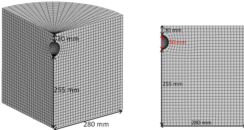
Figure 4.28: Mesh of the semi-infinite solid with a spherical cavity. Left: global view of the mesh. Right: side view of the mesh.
