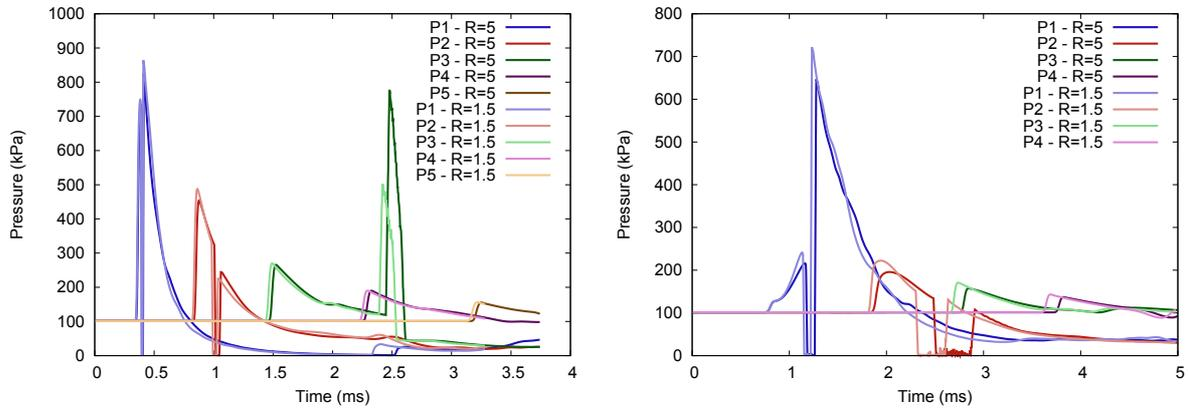
Figure 5.66: Comparison of the pressure profiles at the five outputs for charges buried at 3 cm (left) and at 8 cm (right) for  $R = 1.5$  and  $R = 5$ . The two values of  $R$  provide very close pressure results. For a depth of burial of 8 cm, the differences are much more noticeable than for a depth of burial of 3 cm: the pressure peaks are slightly larger and arrive much earlier with  $R = 1.5$ .
