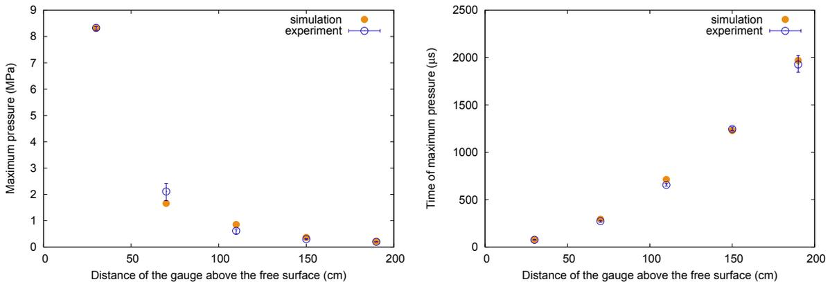
Figure 5.40: Maximum pressures (left) and their respective times (right) at the five outputs for a flush explosive.
