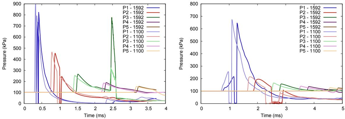
Figure 5.58: Comparison of the pressure profiles at the five outputs for charges buried at 3 cm (left) and 8 cm (right) for  $\rho_0 = 1592$  and  $1100 \text{ kg.m}^{-3}$ . With an initial density of  $1100 \text{ kg.m}^{-3}$ , the pressures are in advance and slightly larger.
