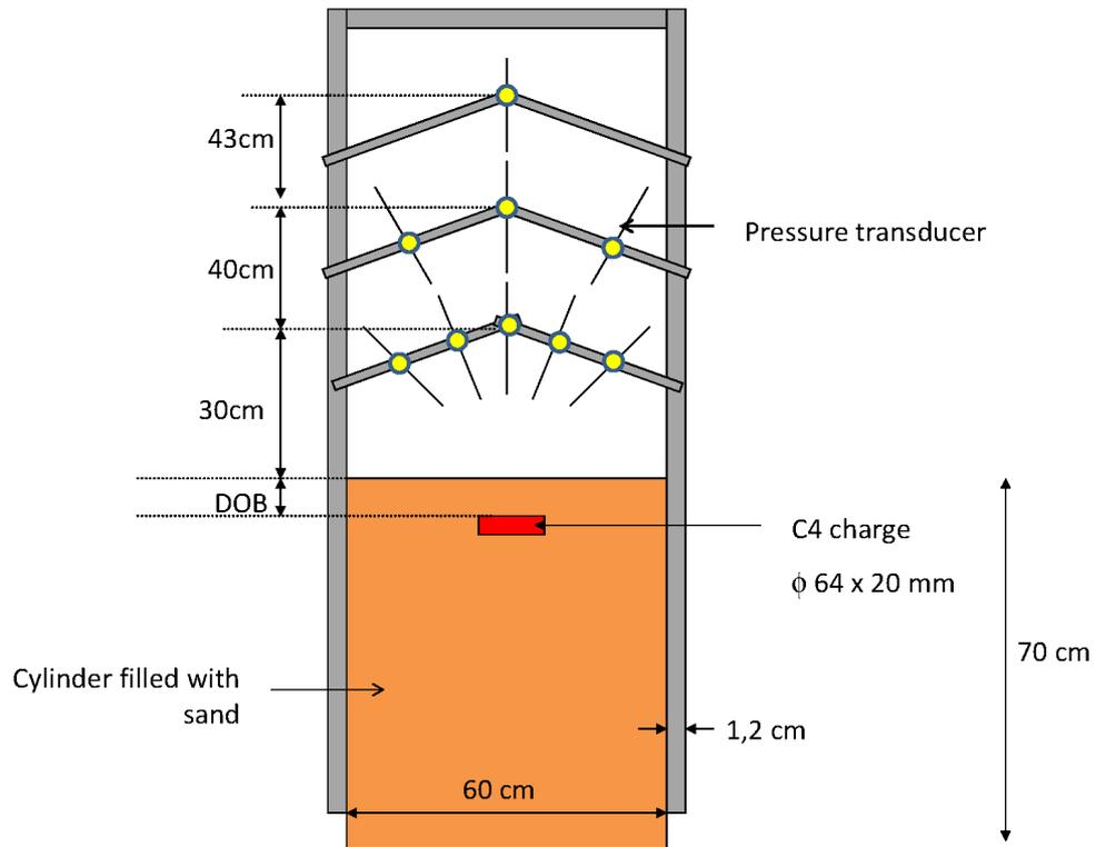
Figure 5.6: Experimental setup used by for Materials Sciences Corporation (2006). The sand was either dry or saturated.
