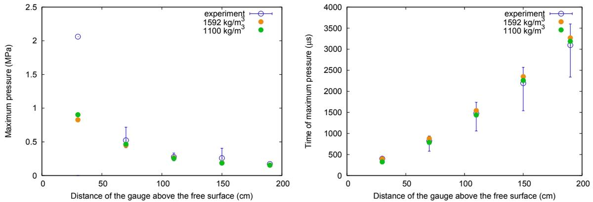
Figure 5.59: Maximum pressures (left) and their respective times (right) at the five outputs for a DOB of 3 cm in experiments, in simulations with initial densities  $\rho_0 = 1592$  and  $1100 \text{ kg.m}^{-3}$ . Except for the first peak, we obtained the closest results to experiments with the smallest density.
