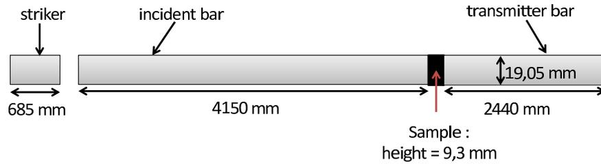
Figure 4.10: SHPB disposal used for the simulations.
