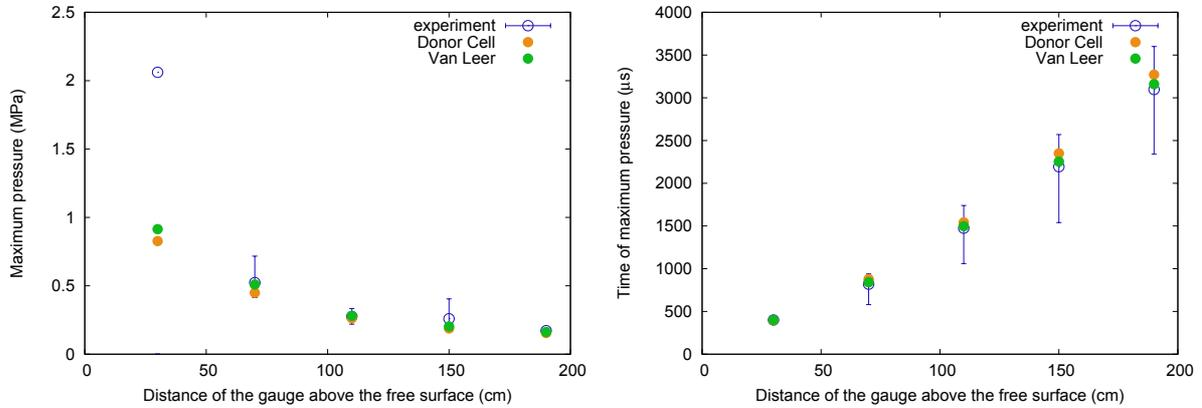
Figure 5.51: Maximum pressures (left) and their respective times (right) at the five outputs for a DOB of 3 cm in experiments, and with the Van Leer and Donor cell algorithms.
