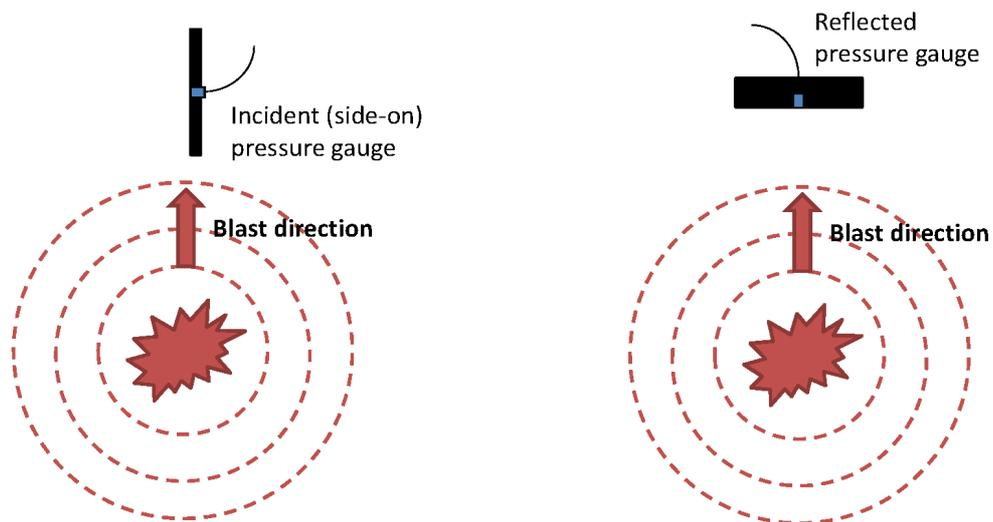
Figure 5.7: Side-on and reflected pressures. If the pressure gauge is parallel to the direction of the shock wave, this is a side-on pressure, whereas if the pressure gauge is embedded in a rigid material perpendicularly to the direction of the shock wave, this is a reflected pressure.
