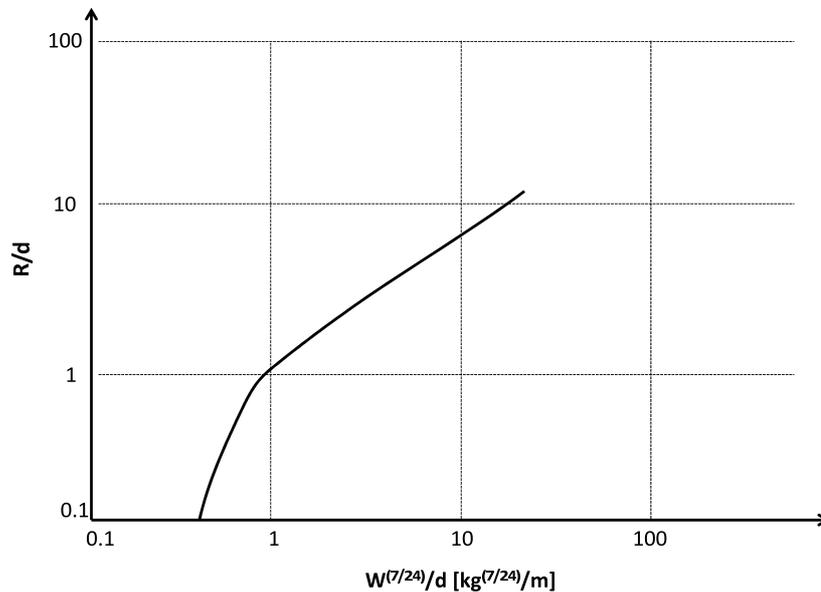
Figure 5.4: Variation of the ratio of the crater radius by the depth of burial of the explosive as a function of the entity proposed by Luccioni and Ambrosini (2006).
