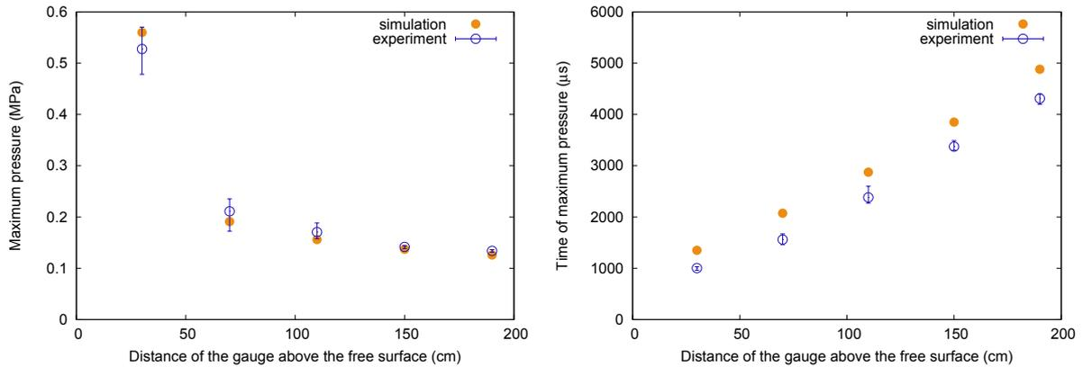
Figure 5.44: Maximum pressures (left) and their respective times (right) at the five outputs for a DOB of 8 cm. All the pressures fit with the experiments. An almost constant time shift exists between the simulations and the experiments. The soil and in particular the upper soil layer was less tamped in the experiments with this depth of burial. Perhaps the density of the soil was smaller which provoked this time shift.
