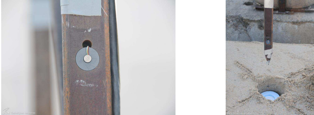
Figure 5.12: Pressure gauges used for the shots with explosives buried at 8 cm. In this case, the pressure gauges are piezoresistive: the resistance of the gauge is modified because of the shock wave which changes the voltage which is linked to the pressure. The edge of the shaft is sharp, so that it does not disturb the propagation of the shock wave.
