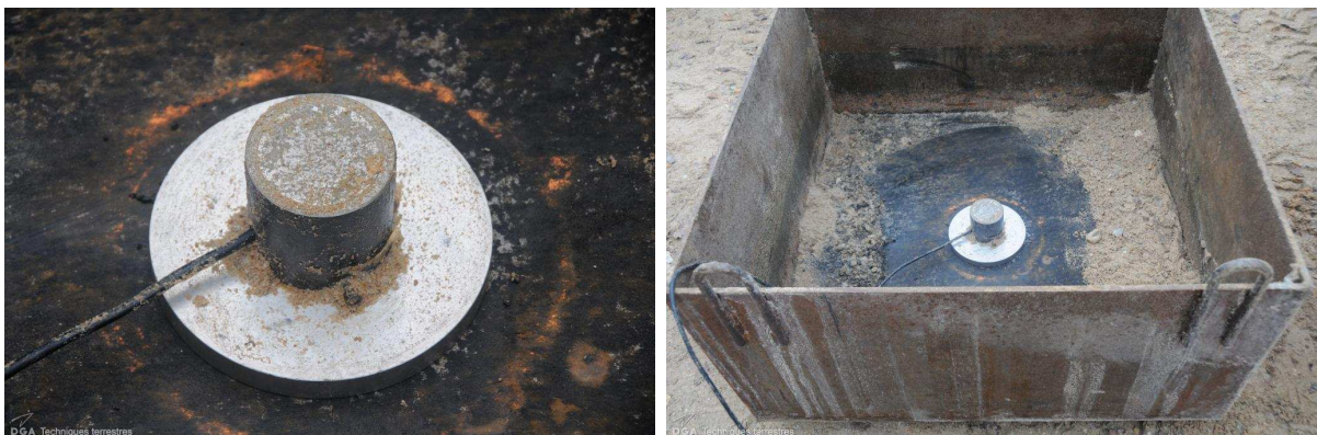
Figure 5.13: The force gauge with a diameter of 70 mm used for the shots in January. This device was placed at the bottom of the soil tank.
