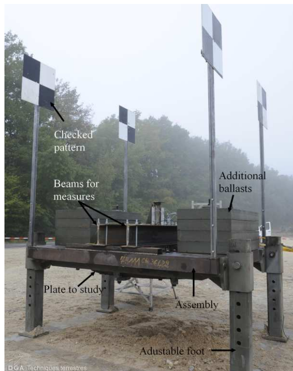
Figure 6.17: View of our large scale experimental set up. The deformation of a metallic plate and the impulse transmitted by buried detonations were studied.
