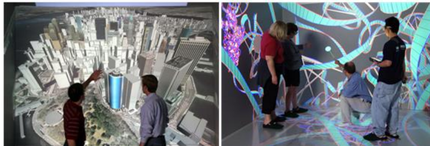
Figure 2-8: The six-channel CAVE system, the 10' x 10' environment features wireless tracking and communication devices and a three-dimensional audio system, IOWA State University [IOWA 2013]
