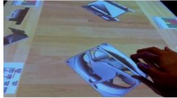
E. Rotation of 3D document: rotation is down based on more than 2 finger interaction and around the center of object with user hand replacement direction
