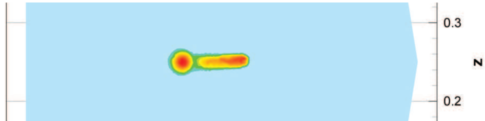
Figure 6.16: Electron density at times t_1 = 1.26 \cdot 10^{-8} s, isolines in a cut plane y = 0.25
