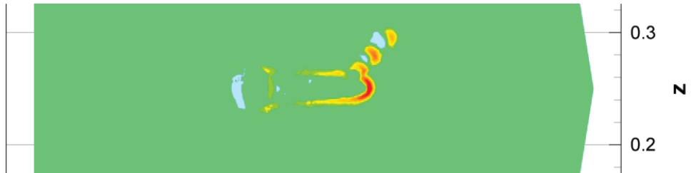
Figure 6.72: Net charge density at times t_1 = 1.36 \cdot 10^{-8} s, isolines in a cut plane y = 0.25
