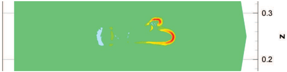
Figure 6.49: Net charge density at times t_1 = 1.47 \cdot 10^{-8} s, isolines in a cut plane y = 0.25
